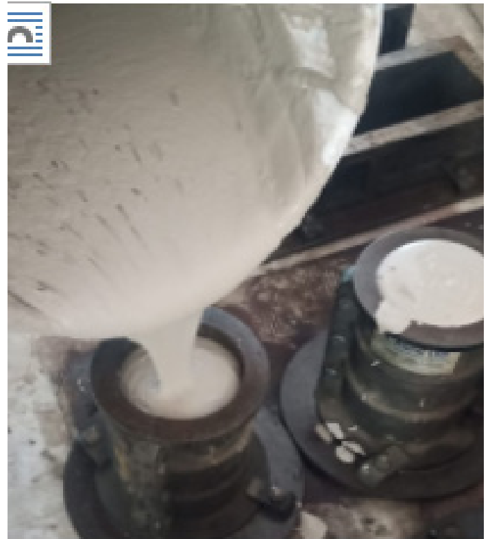
Fig. 2b: Fresh geopolymer foam
