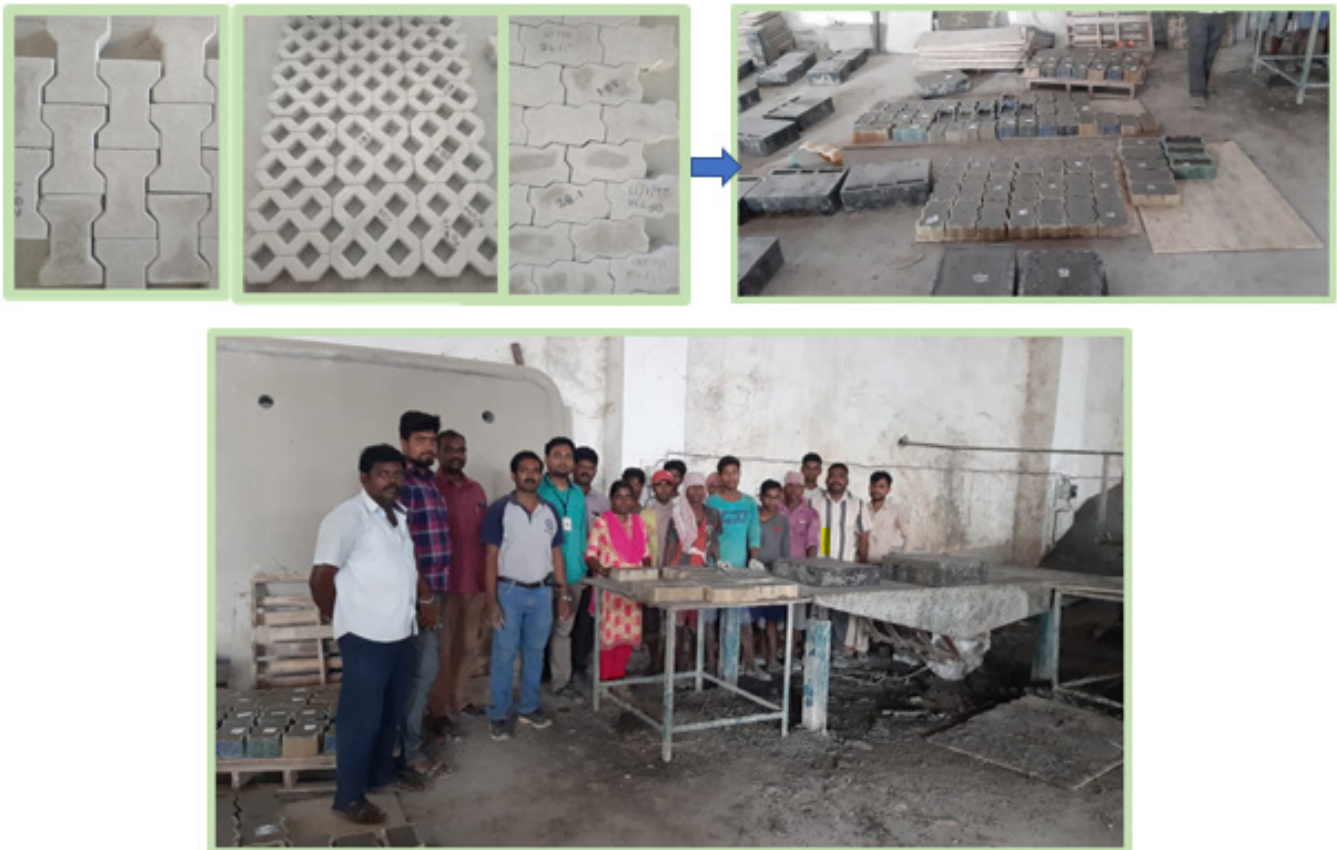
Fig. 1: Pilot scale demonstration of geopolymer paver block technology
