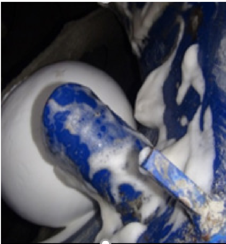
Fig. 2a: A pre-formed mechanical foam
